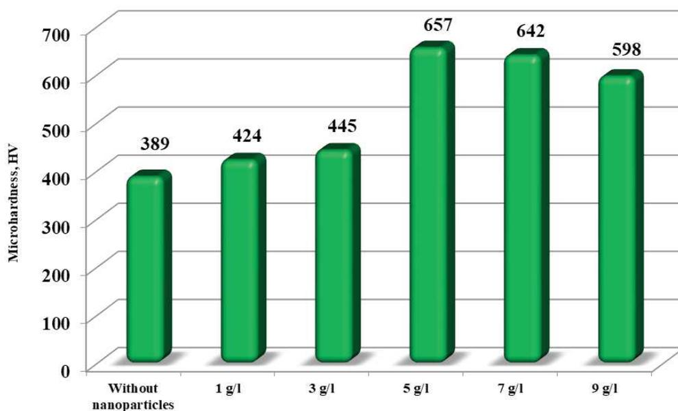
Fig. 4. Histogram of the microhardness of the nanocomposite zinc coating depending on the concentration of nanosized particles in the electrolyte
