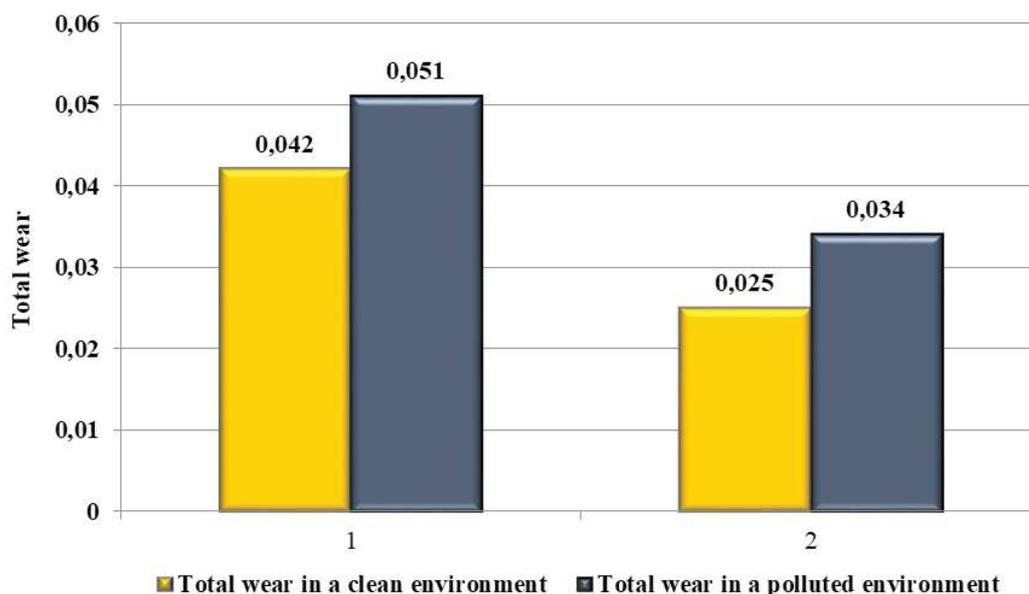
Fig. 5. Total wear of friction pairs with zinc coating after wear resistance tests: 1 - without adding nanosized particles; 2 - with the addition of nanosized  $Al_2O_3$  particles
