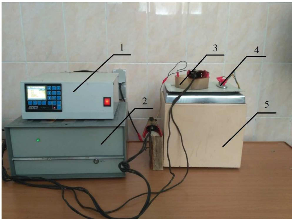
*Fig. 1. Laboratory galvanic equipment: 1 – rectifier GTP 500 – 30 (5) x12R – 220 – P2 / B2; 2 – power supply unit for the ultrasonic bath; 3 – electrolyte container; 4 – heating element; 5 – ultrasonic bath*
