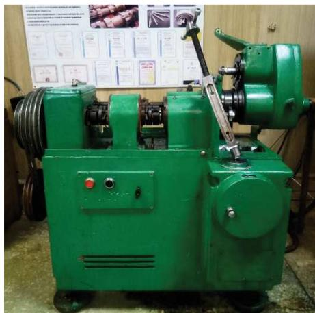
Fig. 2. Friction machine SMTs-2
