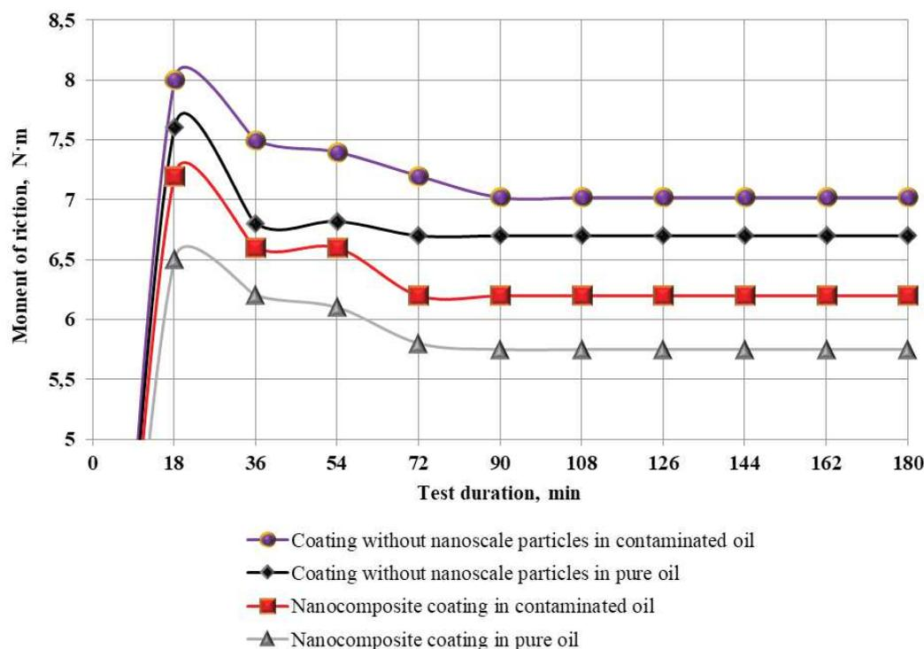
Fig. 6. Change in friction moment during wear resistance tests
